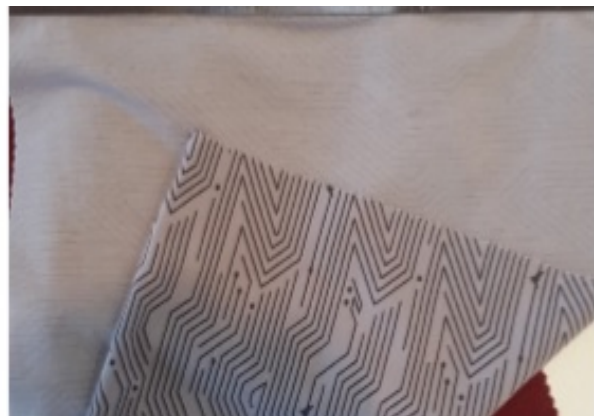
Polyester, wool and elastane blend jersey fabric with graphene print by Movetec
